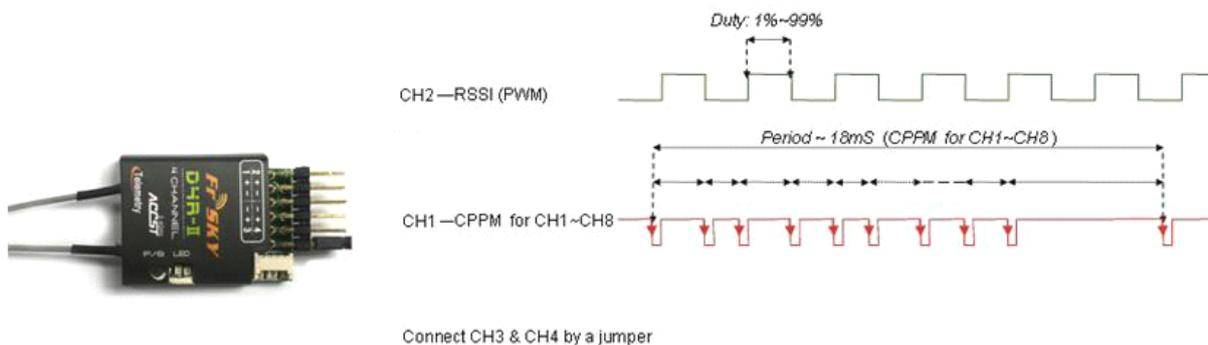
**CPPM channel can not handle all eight channels at the same time with all throws are maxed out, as it does not have enough frame gap. It is recommended to use at most six channels from CPPM channel while leaving off the rest two channels, otherwise improper performance might occur.**
