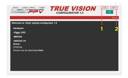
**STEP 4:** Plug Battery for Kombini DS, then click **Connect icon** on True Vision interface to connect and configuration OSD layout and setting.
